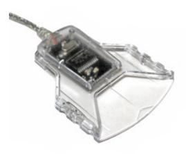
The IDBridge CT30 (formerly the GemPC Twin/TR) USB desktop reader from Gemalto integrates high quality and functionality with a contemporary design. This reader is fully PC/SC and EMV Level 1 compliant and supports all ISO 7816 microprocessor-based smartcards as well as many popular memory cards. The reader is compatible with previous Gemalto models such as the GCR410.
